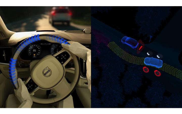
This system helps the driver take evasive action in an emergency situation. If the driver faces a vehicle, a cyclist, a pedestrian, or a large animal in front, braking is not always enough – steering away is sometimes necessary to avoid an accident.
