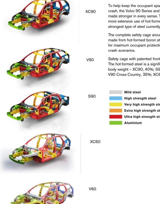
To help keep the occupant space inside intact in a crash, the Volvo 90 Series and 60 Series cars are made stronger in every sense. This is achieved with a more extensive use of hot-formed boron steel, the strongest type of steel currently used in the car industry.
