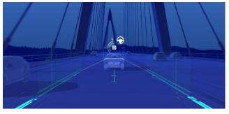
The driver can override the system at any time by using the brake pedal, accelerator pedal or steering wheel. Using the turn indicator will temporarily abort the steering support if the driver wants to change lane.
